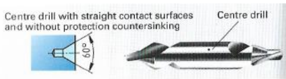
Figure 3: Centring drill hole with centring drill Source: BARTENSCHLAGER ET AL. (2016, p. 144).
